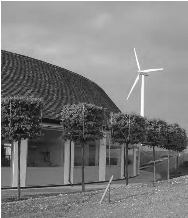
17.2 Boxed hornbeams provide solar shading.
